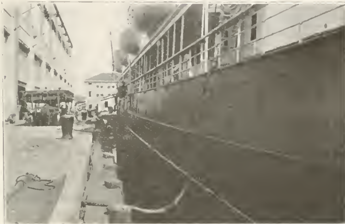
Unguarded water hose are a constant source of danger. They should be disconnected or rat-guarded when not in use.
